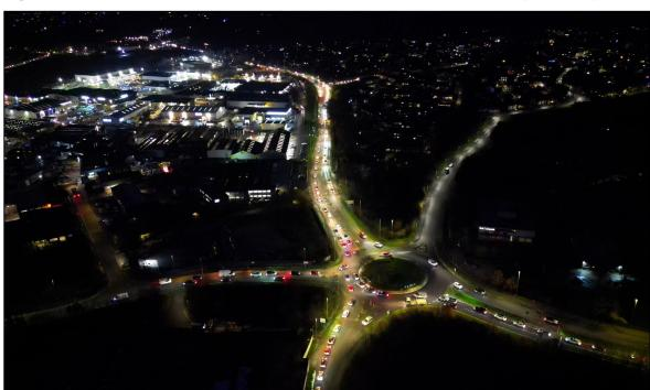
Figure 5.11: Observed Queues on A28 SB Back to Tank Roundabout (PM Peak)
